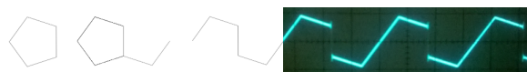
Figure 1: An n-gon wave is derived from a pentagon. The internal angle of 3\pi/5 rad of the pentagon is retained in the shape of the wave and in the visualisation of the resulting pentagon wave on a cathode-ray oscilloscope.
