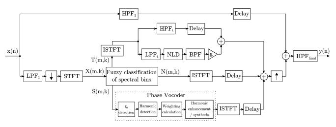
Figure 3: Proposed virtual bass algorithm in which the transient part T(m, k) is processed in a different way than the tonal part S(m, k).
