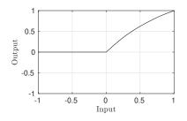
Figure 4: *HWR-FEXP1* transfer function is a combination of a half-wave rectifier and an exponential function.
